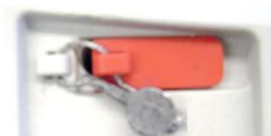
Locked with Wire Seal
