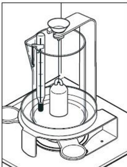
Suspend the sinker (8) from the bracket and ensure that it does not touch either the beaker or the thermometer.
