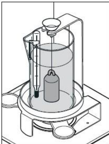
Add the liquid whose density you wish to determine to the beaker (up to approx. 1 cm above the suspension eye of the sinker). Ensure that no air bubbles adhere to the sinker (remove any air bubbles with a fine brush).
