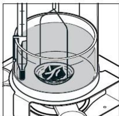
Place the solid after in the holder (6). Ensure that no air bubbles adhere to the solid (remove any air bubbles with a fine brush).
