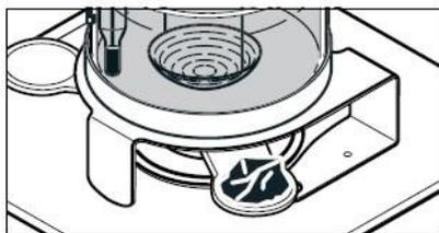
Place the solid in one of the two weighing pans of the bracket (2). Wait until the weight display of the balance is stable and note the displayed weight A (weight of sample in air).
