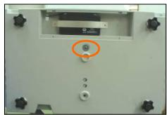
5.9. Place the 15 kg dead weight on the backhand side of the scales on the scale indicator 15kg will appear, tighten the upper screw until 14kg appears on the indicator and close the nut.
