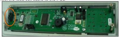
4.9. Attach back the RFI to the PCB, Make sure the load cell cable is not pinch between the RFI box and the PCB.
