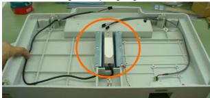
3.10. Fasten plastic fasteners to attach the LC cable to the housing.
