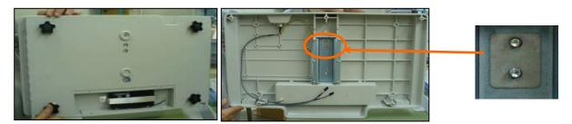
3.9. Ensure that the Load Cell is placed parallel to its housing and tighten the base Load cell screws using a torque gauge at 13 NM.
