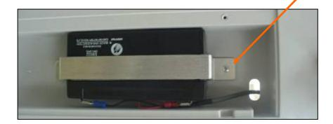
1.7. Put the cover back in place and fasten by screwing in two Philips M3X6 (401426) screws.
