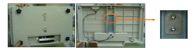
3.7. Cut the cable fasteners which connect the load cell to the housing
