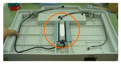
3.6. Turn the base on its side and unscrew two allen screws M6X16 (400659) releasing two washers M6 (404075) and the metal spacer of 2mm (590320)) from the lower Load Cell housing, keep for reassembly.
