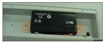
1.6. Place the battery fastener over the battery and screw it into place using two Philips screws M3X6 (401426).
