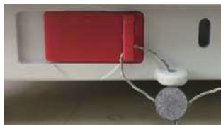
Locked with Wire Seal
